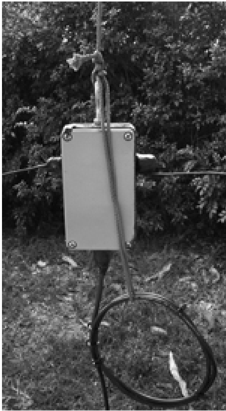
Balun – the cord takes the weight and the sealing tape keeps the weather out
