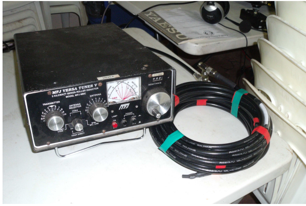
The roll of 213 coaxial cable is a tuning stub
