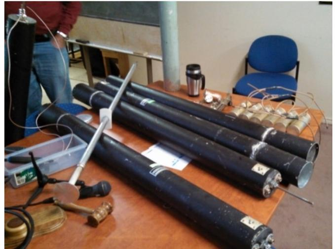
An example of the filter types is shown alongside. These included 6 metre to 470 MHz and higher cavity filters. (note the coffer transport container was non-resonant at all test frequencies).
